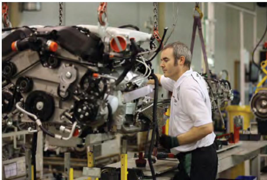
Figure 23.5: Job production – every Aston Martin engine is built by hand
